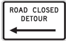
Road is closed. The arrow points in the direction of the detour.
