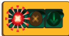
Control signal: Placed over lanes to indicate which ones are open for driving. Here: RED = do not drive in Right lane.
